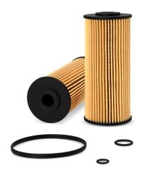
Largest OD68.07 mmLargest End ID17.02 mmLength155.65 mmFlow DirectionOutside InGasket Inside Diameter17.02 mm
