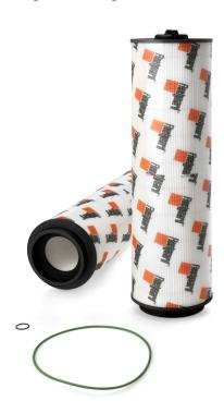
Media TypeMicroglassBPV OPENING DPNoLargest End ID78.23 mmLargest OD152.40 mmLength550.67 mmGasket Inside Diameter117.07 mm
