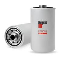
**Thread Size** M42 X 2-6H INT **BPV OPENING DP** 28 kPa Length 259.00 mm Seam OD 137.00 mm TWA MICRON @ BETA=2 11 micron TWA MICRON @ BETA=20 25 micron TWA MICRON @ BETA=200 39 micron TWA MICRON @ BETA=75 33 micron
