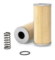
End 1 ID 41.00 mm **BPV OPENING DP** 240 kPa 95.00 mm Largest OD End 2 OD 95.00 mm Length 292.00 mm TWA MICRON @ BETA=2 35 micron TWA MICRON @ BETA=20 60 micron TWA MICRON @ BETA=75 75 micron
