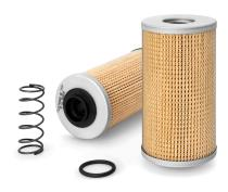
End 1 ID 29.00 mm End 2 OD 70.00 mm **BPV OPENING DP** 250 kPa 70.00 mm Largest OD Length 196.00 mm TWA MICRON @ BETA=2 35 micron TWA MICRON @ BETA=20 60 micron TWA MICRON @ BETA=75 75 micron
