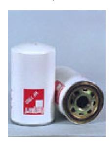
**BPV OPENING DP** Yes **Thread Form** British 227.50 mm Length Largest OD 128.00 mm **Gasket Inside Diameter** 98.00 mm 106.50 mm **Gasket OD** 1500 kPa **Hydrostatic Burst Minimum** Particle Size at Beta 75 10 micron **Thread Type** Internal
