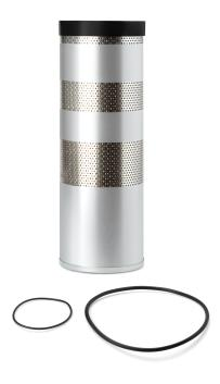
439.00 mm Length 98.00 mm Largest End ID 154.00 mm Largest OD **BPV OPENING DP** No **Gasket Inside Diameter** 112.50 mm Gasket OD 130.00 mm Particle Size at Beta 75 45 micron Flow Direction Outside In
