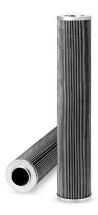
Length 428.24 mm End 2 OD 78.99 mm Largest OD 79.25 mm 42.42 mm End 2 ID **BPV OPENING DP** 0 kPa TWA MICRON @ BETA=20 1 micron TWA MICRON @ BETA=200 5 micron TWA MICRON @ BETA=75 3 micron
