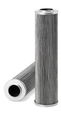
End 2 ID 42.42 mm **BPV OPENING DP** 0 kPa Length 328.68 mm End 2 OD 78.99 mm 79.25 mm Largest OD TWA MICRON @ BETA=2 4 micron TWA MICRON @ BETA=20 9 micron TWA MICRON @ BETA=200 14 micron TWA MICRON @ BETA=75 12 micron
