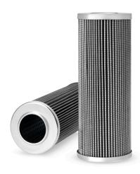
End 2 OD 78.99 mm 79.25 mm Largest OD **BPV OPENING DP** 0 kPa 208.03 mm Length End 2 ID 42.42 mm TWA MICRON @ BETA=2 9 micron TWA MICRON @ BETA=20 19 micron TWA MICRON @ BETA=200 30 micron TWA MICRON @ BETA=75 25 micron
