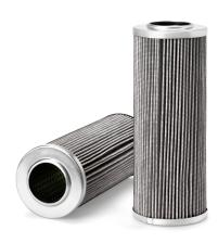
Length 208.03 mm **BPV OPENING DP** 0 kPa 79.25 mm Largest OD End 2 ID 42.42 mm End 2 OD 78.99 mm TWA MICRON @ BETA=2 4 micron TWA MICRON @ BETA=20 9 micron TWA MICRON @ BETA=200 14 micron TWA MICRON @ BETA=75 12 micron
