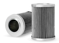
End 2 OD 78.99 mm 117.60 mm Length **BPV OPENING DP** 0 kPa End 2 ID 42.42 mm Largest OD 79.25 mm TWA MICRON @ BETA=2 9 micron TWA MICRON @ BETA=20 19 micron TWA MICRON @ BETA=200 30 micron TWA MICRON @ BETA=75 25 micron
