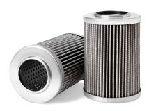
Length 117.60 mm End 2 OD 78.99 mm **BPV OPENING DP** 0 kPa 79.25 mm **Largest OD** End 2 ID 42.42 mm TWA MICRON @ BETA=20 4 micron TWA MICRON @ BETA=200 8 micron TWA MICRON @ BETA=75 6 micron
