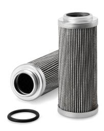
Length 113.54 mm End 2 ID 24.89 mm 45.21 mm Largest OD End 2 OD 44.45 mm TWA MICRON @ BETA=2 9 micron TWA MICRON @ BETA=20 19 micron TWA MICRON @ BETA=200 30 micron TWA MICRON @ BETA=75 25 micron
