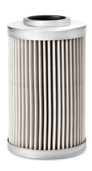
Largest OD 69.00 mm 33.20 mm End 1 ID 116.00 mm Length End 2 OD 69.00 mm TWA MICRON @ BETA=2 4 micron TWA MICRON @ BETA=20 6 micron TWA MICRON @ BETA=200 12 micron TWA MICRON @ BETA=75 10 micron
