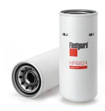
**Thread Size** 1 1/2-16 UN-2B Length 297.94 mm 124.33 mm Largest OD **BPV OPENING DP** 0 kPa **Gasket Inside Diameter** 90.80 mm Gasket OD 104.27 mm Seam OD 125.73 mm **Standpipe** NO TWA MICRON @ BETA=2 6 micron TWA MICRON @ BETA=20 15 micron TWA MICRON @ BETA=200 24 micron TWA MICRON @ BETA=75 20 micron
