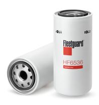
Largest OD93.47 mmThread Size3/4-14 BSPLength205.49 mmGasket Inside Diameter62.53 mmGasket OD71.98 mmSeam OD94.44 mmStandpipeNO
