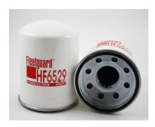
Length 175.00 mm **Thread Diameter** 48.00 mm Thread Pitch 2.00 mm **Largest OD** 133.50 mm **Thread Form** Metric **Gasket Inside Diameter** 115.00 mm **Gasket OD** 124.50 mm **Hydrostatic Burst Minimum** 1500 kPa Thread Class None Thread Type Internal Flow Direction Outside In
