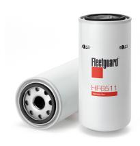
Largest OD 93.47 mm 1-12 UNF-2B **Thread Size** 205.49 mm Length **BPV OPENING DP** 0 kPa Seam OD 94.49 mm **Gasket Inside Diameter** 62.48 mm **Gasket OD** 71.88 mm NO **Standpipe** TWA MICRON @ BETA=2 16 micron TWA MICRON @ BETA=20 35 micron 47 micron TWA MICRON @ BETA=75
