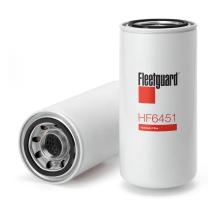
Largest OD93.73 mmLength222.50 mmGasket Inside Diameter62.74 mmGasket OD72.14 mmHydrostatic Burst Minimum2068 kPa
