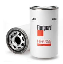
231.00 mm Length 132.00 mm Largest OD **Thread Form** British **BPV OPENING DP** No **Gasket Inside Diameter** 98.00 mm **Gasket OD** 108.00 mm **Hydrostatic Burst Minimum** 1500 kPa Particle Size at Beta 75 75 micron Internal Thread Type
