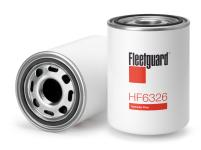
181.50 mm Length **Thread Form** British 130.00 mm Largest OD **BPV OPENING DP** Yes **Gasket Inside Diameter** 97.00 mm 106.50 mm **Gasket OD Hydrostatic Burst Minimum** 1500 kPa Particle Size at Beta 75 35 micron Flow Direction Outside In
