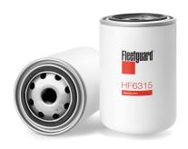
Thread Size 3/4-16 UNF-2B Length 142.50 mm **Largest OD** 93.50 mm **BPV OPENING DP** 250 kPa **Gasket Inside Diameter** 62.00 mm **Gasket OD** 70.00 mm Seam OD 93.50 mm Standpipe NO TWA MICRON @ BETA=2 33 micron TWA MICRON @ BETA=20 55 micron TWA MICRON @ BETA=75 65 micron
