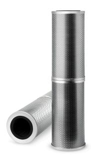
88.00 mm Largest End ID 152.00 mm Largest OD **BPV OPENING DP** No Length 624.00 mm **Gasket Inside Diameter** 90.00 mm **Gasket OD** 110.00 mm Particle Size at Beta 75 20 micron Flow Direction Inside Out
