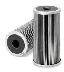
**BPV OPENING DP** 0 kPa End 2 OD 114.55 mm 226.82 mm Length End 1 ID 36.58 mm 114.55 mm Largest OD End 2 ID 36.58 mm TWA MICRON @ BETA=2 4 micron TWA MICRON @ BETA=20 9 micron TWA MICRON @ BETA=75 12 micron
