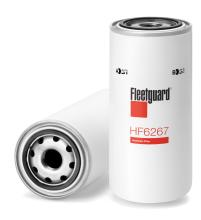
Thread Size 1-12 UNF-2B Largest OD 93.50 mm 210.10 mm Length **BPV OPENING DP** 250 kPa **Gasket Inside Diameter** 62.00 mm Gasket OD 70.00 mm Seam OD 93.50 mm NO **Standpipe** TWA MICRON @ BETA=2 20 micron TWA MICRON @ BETA=20 30 micron TWA MICRON @ BETA=75 35 micron
