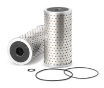
114.55 mm Largest OD End 2 ID 36.58 mm **BPV OPENING DP** 0 kPa End 1 ID 36.58 mm Length 226.31 mm 114.55 mm End 2 OD 2 micron TWA MICRON @ BETA=2 TWA MICRON @ BETA=20 8 micron TWA MICRON @ BETA=75 13 micron
