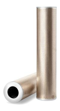
End 2 OD 101.35 mm End 1 ID 56.64 mm 101.60 mm Largest OD 0 kPa **BPV OPENING DP** 456.18 mm Length TWA MICRON @ BETA=2 16 micron TWA MICRON @ BETA=20 35 micron TWA MICRON @ BETA=75 47 micron
