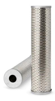
End 1 ID 25.40 mm Length 277.88 mm Largest OD 64.01 mm **BPV OPENING DP** 0 kPa End 2 OD 64.01 mm End 2 ID 25.40 mm TWA MICRON @ BETA=2 12 micron TWA MICRON @ BETA=20 27 micron TWA MICRON @ BETA=75 35 micron
