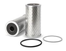
End 1 ID 36.58 mm End 2 OD 114.55 mm 114.55 mm Largest OD End 2 ID 36.58 mm Length 226.31 mm **BPV OPENING DP** 0 kPa TWA MICRON @ BETA=2 2 micron TWA MICRON @ BETA=20 8 micron TWA MICRON @ BETA=75 13 micron
