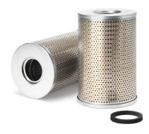
114.81 mm Largest OD End 2 ID 45.72 mm 177.80 mm Length End 2 OD 114.81 mm End 1 ID 45.72 mm **BPV OPENING DP** 0 kPa TWA MICRON @ BETA=2 26 micron TWA MICRON @ BETA=20 41 micron
