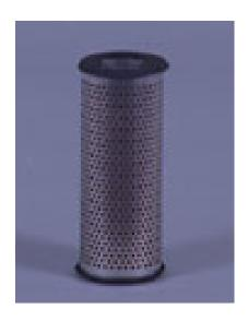
59.18 mm Largest OD End 2 OD 59.18 mm End 1 ID 34.54 mm 0 kPa **BPV OPENING DP** End 2 ID 34.54 mm 152.65 mm Length TWA MICRON @ BETA=2 22 micron TWA MICRON @ BETA=20 43 micron
