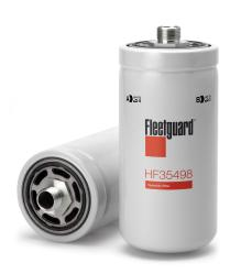
24.00 mm **Thread Diameter** Thread Pitch 1.50 mm **BPV OPENING DP** No Thread Form Metric 95.25 mm Largest OD Length 219.96 mm **Gasket Inside Diameter** 63.09 mm Gasket OD 70.15 mm 6895 kPa **Hydrostatic Burst Minimum** Particle Size at Beta 200 21.0 Particle Size at Beta 75 20.0 **Thread Class** 6G Flow Direction Outside In
