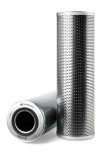
**BPV OPENING DP** No 372.00 mm Length **Largest OD** 116.00 mm Largest End ID 56.00 mm **Gasket Inside Diameter** 65.00 mm **Gasket OD** 80.00 mm Particle Size at Beta 75 20 micron Flow Direction Inside Out
