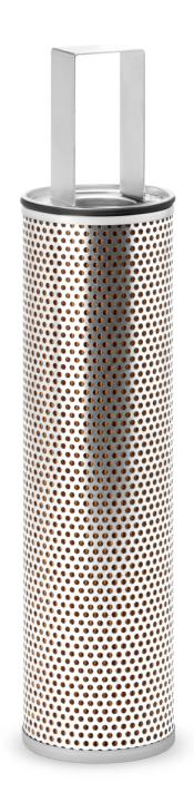
84.50 mm **Largest OD** 18.00 mm End 2 ID Length 304.00 mm End 1 ID 40.00 mm End 2 OD 83.50 mm **BPV OPENING DP** 30 kPa TWA MICRON @ BETA=2 35 micron TWA MICRON @ BETA=20 60 micron **TWA MICRON @ BETA=75** 75 micron
