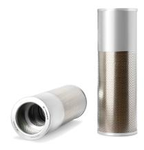
Length450.00 mmBPV OPENING DPNoLargest End ID85.00 mmLargest OD150.00 mmParticle Size at Beta 7550 micronFlow DirectionOutside In
