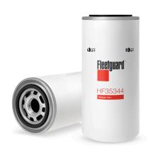
Length 210.50 mm 96.50 mm Largest OD **BPV OPENING DP** No **Thread Form** British Gasket Inside Diameter 62.00 mm Gasket OD 71.00 mm **Hydrostatic Burst Minimum** 1500 kPa Particle Size at Beta 200 8 micron Particle Size at Beta 75 5 micron Internal **Thread Type** Flow Direction Outside In
