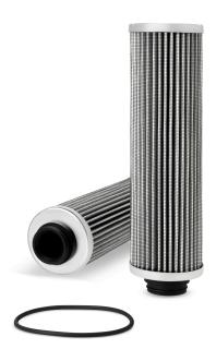
244.50 mm Length **BPV OPENING DP** No 67.00 mm Largest OD 25.00 mm Largest End ID Gasket OD 37.00 mm Particle Size at Beta 200 12 micron Particle Size at Beta 75 10 micron Flow Direction Outside In
