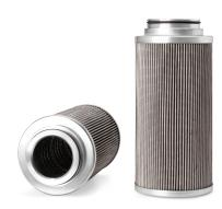
47.50 mm Largest End ID **BPV OPENING DP** No 93.50 mm Largest OD Length 200.00 mm **Gasket OD** 64.50 mm Particle Size at Beta 200 12 micron Particle Size at Beta 75 10 micron Outside In Flow Direction
