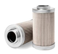
Length85.00 mmLargest OD47.00 mmBPV OPENING DPNoLargest End ID22.00 mmGasket Inside Diameter22.00 mmParticle Size at Beta 7520 micronFlow DirectionOutside In
