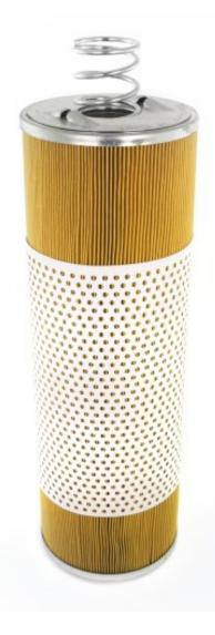
Largest OD130.00 mmLargest End ID85.50 mmGasket Inside Diameter90.00 mmParticle Size at Beta 7575 micronFlow DirectionOutside In
