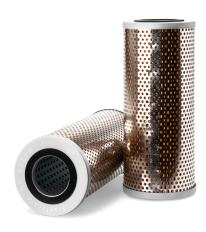
Largest End ID 40.50 mm **BPV OPENING DP** No **Largest OD** 83.00 mm 197.50 mm Length **Gasket Inside Diameter** 43.00 mm Gasket OD 57.00 mm Particle Size at Beta 75 45 micron Flow Direction Outside In
