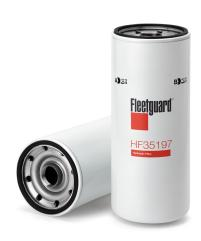
Largest OD107.67 mmThread Size1 1/8-16 UN-2BLength263.91 mmBPV OPENING DP0 kPaGasket Inside Diameter90.55 mmGasket OD99.95 mm
