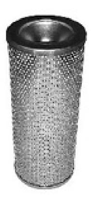
**BPV OPENING DP** No Length 260.00 mm Largest End ID 72.00 mm Largest OD 106.00 mm Gasket Inside Diameter 9.93 mm Particle Size at Beta 200 4 micron Particle Size at Beta 75 3 micron **Flow Direction** Inside Out
