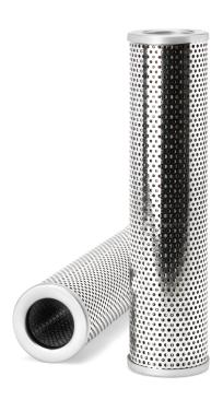
**BPV OPENING DP** No Length 300.00 mm Largest End ID 45.00 mm Largest OD 72.00 mm Gasket Inside Diameter 7.60 mm Particle Size at Beta 200 12 micron Particle Size at Beta 75 10 micron Flow Direction Inside Out
