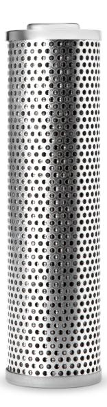
231.00 mm Length Largest End ID 29.00 mm **BPV OPENING DP** No 64.00 mm Largest OD **Gasket Inside Diameter** 26.57 mm Particle Size at Beta 200 12 micron Particle Size at Beta 75 10 micron Flow Direction Inside Out
