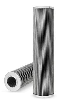
End 2 OD 78.99 mm **Largest OD** 79.25 mm Length 328.93 mm End 2 ID 42.42 mm TWA MICRON @ BETA=2 5 micron TWA MICRON @ BETA=20 12 micron TWA MICRON @ BETA=200 25 micron TWA MICRON @ BETA=75 15 micron
