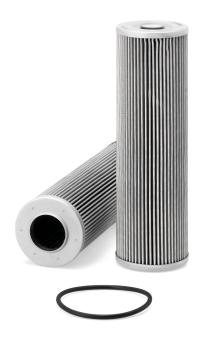
Largest End ID 48.50 mm 322.00 mm Length **BPV OPENING DP** No 94.00 mm Largest OD **Gasket Inside Diameter** 47.00 mm Particle Size at Beta 200 25 micron Particle Size at Beta 75 15 micron Flow Direction Outside In
