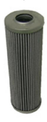
**BPV OPENING DP** No Largest OD 73.00 mm 32.00 mm Largest End ID Length 236.00 mm **Gasket Inside Diameter** 31.50 mm Particle Size at Beta 200 25 micron Particle Size at Beta 75 15 micron Flow Direction Outside In
