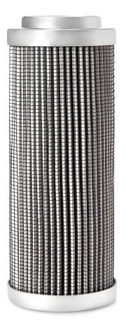
End 2 OD End 2 ID Length Largest OD TWA MICRON @ BETA=2 TWA MICRON @ BETA=20 44.45 mm 24.89 mm 113.54 mm 45.21 mm 5 micron 12 micron 25 micron 15 micron
